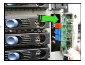
4. Remove the screw that secures the I/O board to the bracket.
